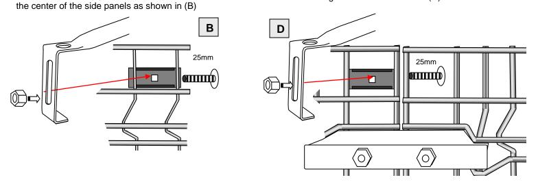
Install the straight ridge line braces using the clamps provided. Adjust the distance between the trusses so they are vertical by moving the brace in or out of the clamps before tightening the bolts. Use care that the straight brace is inserted at least past the round hole.
