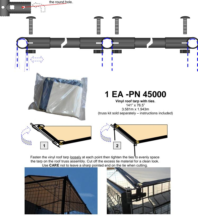
**Caution:** Kennels with roofs or tarps installed should be <u>anchored</u> to prevent them from being overturned in high winds. The roof is **not** designed for heavy snow loads.
